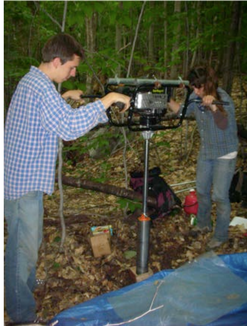
Cores being excavated using a rotary coring device at the Bartlett Experimental Forest (Bartlett, NH).
