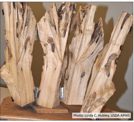
Tabletop display showing internal damage caused by Asian longhorned beetle development within the tree.
